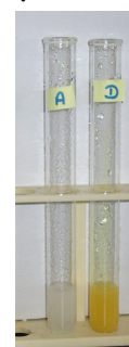
FIGURE 10. Yellow precipitate is shown only in the Sample D with K 3 [Fe(CN) 6 ] solution.
